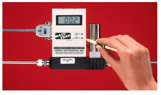
exceptional mass flow control capabilities at a lower cost than any other thermal mass flow controller. Available in any range from 0-10 sccm to 0-50 slpm, the instrument is suitable for any clean, non-corrosive gas flow control application.
