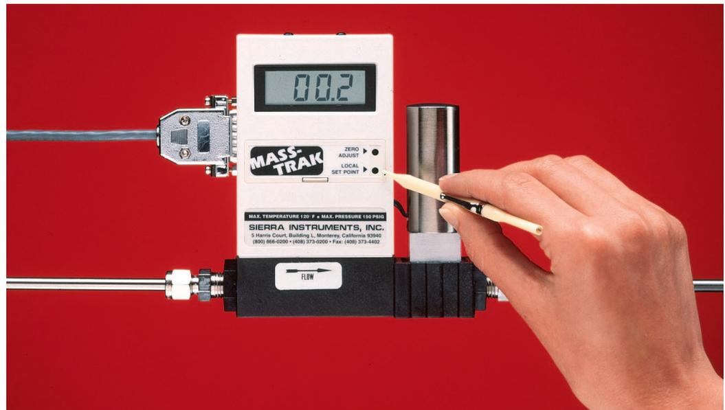
exceptional mass flow control capabilities at a lower cost than any other thermal mass flow controller. Available in any range from 0-10 sccm to 0-50 slpm, the instrument is suitable for any clean, non-corrosive gas flow control application.
