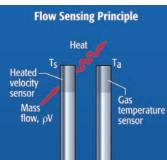
RTD sensor and heater RTD sensor
